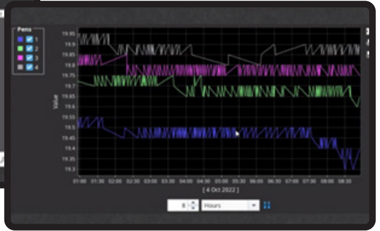
Trends of record temperatures for installed sensors – ability to adjust the historical time frame and also select individual sensor values
